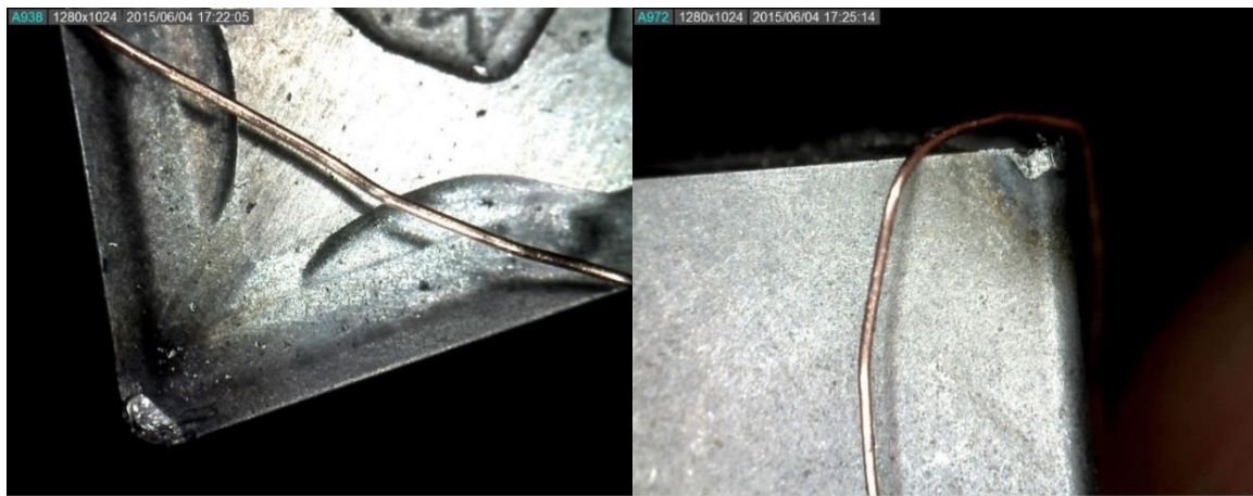
Figure 26. Measurement of the flank and crater wear of the cutting tool using the known electrical wire diameter as reference.
