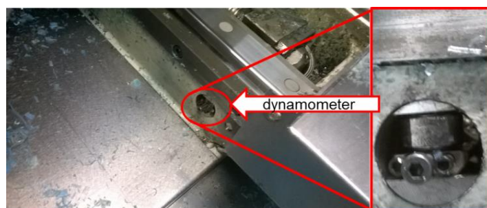
Figure 4. Location of force sensor in drilled pocket
