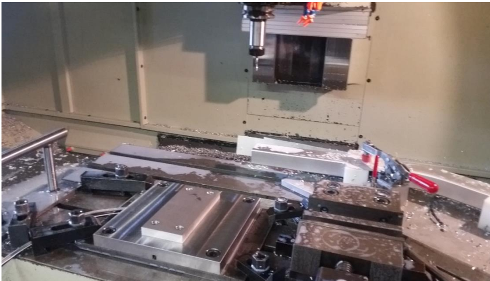
Figure 31. Set-Up fixed on the CNC machine table
