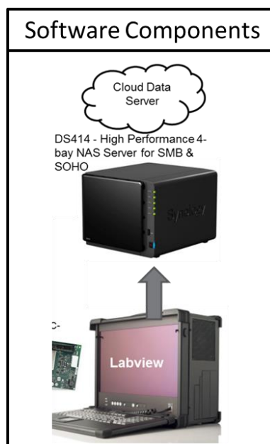
Figure 6. Industrial PC hosting LabView and cloud server.
