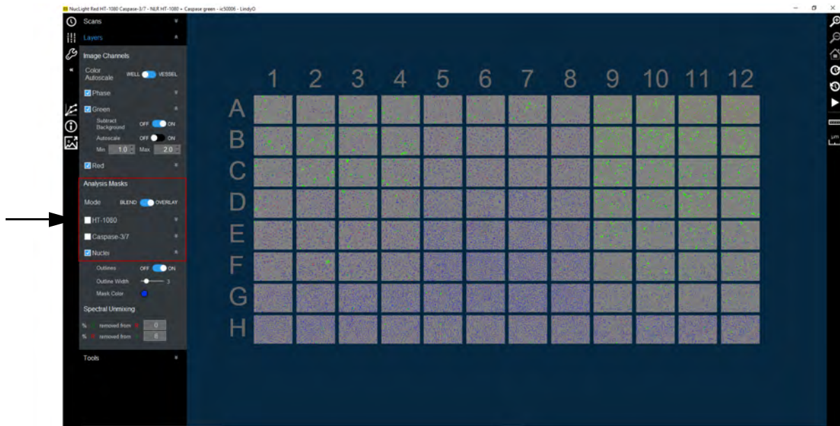
Figure 2-1: Vessel View window with the associated analysis, toggling image masks on and off
